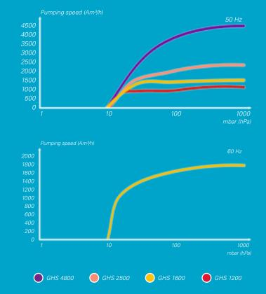
Pump performance measured at the inlet pressure and 20°C. Accuracy is  $^{ au\!/\!-}$  10%.
