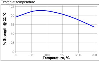
Heat Aging Aged at temperature indicated and tested @ 22 °C
