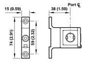
4314-52 - For use with W74 Use 6 mm (7/32") screws to mount bracket to wall.
