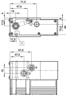
$\fbox{1}$  Valves are delivered with M4 x 50 mounting screws
